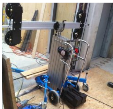
CA 400 GL With cradle for vertical lifting and 2 outriggers for glass up to 4 m
