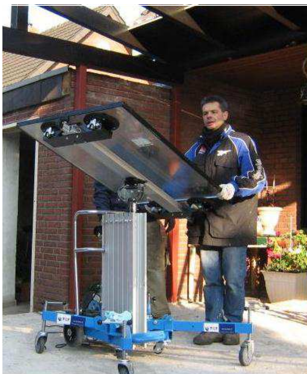
CA 400 GL With cradle for vertical lifting and 2 outriggers for glass up to 4 m
