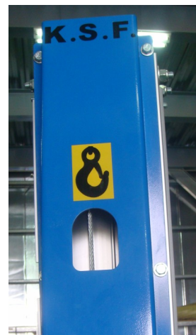
Cable under steel crankbase and crane lifting point for safe transportation
